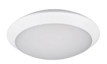
• LED exterior surface mounted luminaire, 350mm diameter, 1500lm as max. lumen output, 17W max. power consumption, 88lm/W efficacy, 4000K color temperature, CRI80, IP66, IK10, 50,000 hours (L70), whitehousing, vandal resistant. Integrated emergency, 3 hours, supplied with anti-theft screws
